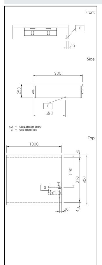
Gas Gas Power: 34 kW Gas Type Option: Gas Inlet: 1/2" **Key Information:** External dimensions, Width: 1000 mm External dimensions, Depth: 900 mm External dimensions, Height: 250 mm Net weight: 82 kg Configuration: Two-Side Operated;Top Front Burners Power: 8.5 - 8.5 kW **Back Burners Power:** 8.5 - 8.5 kW **Back Burners Dimension -**Ø 70 Ø 70
